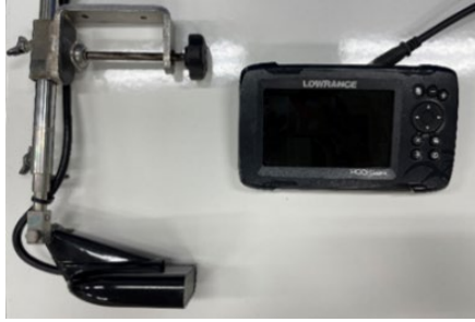
Fig. 2 The underwater ultrasonic sensor used in the study
