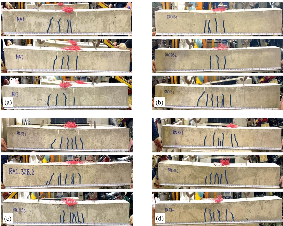
Fig.10 Crack patterns of experimental beams (a) NAC beams, (b) RAC0B beams, (c) RAC30B beams, and (d) RAC70B beams
