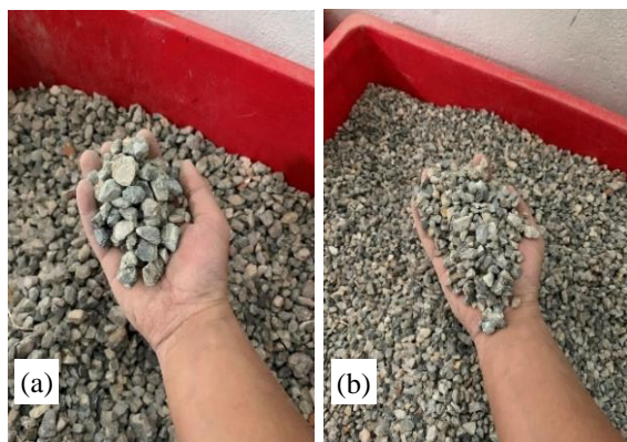
Fig.1 RCA produced from CC of size (a) 10-20mm, and (b) 5-10mm
