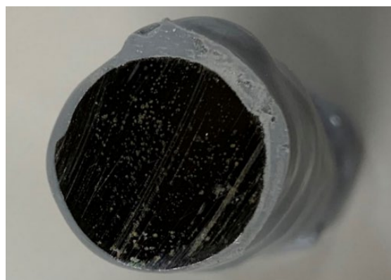
Fig. 2 The photograph of the cut surface of rebar coated with epoxy resin.
