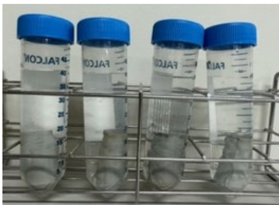
Fig. 3 Experimental setup for the measurement of corrosion amount of rebar immersed in sugar solutions. From left to right: Control Sample, Glucose, Fructose, and WS.
