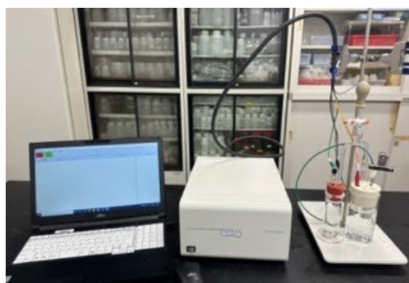
Fig. 4 Experimental setup for Tafel extrapolation.
