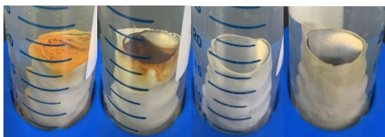
Fig. 5 Surface of rebars immersed in various solutions for one week. From left to right: Control Sample, Glucose, Fructose, and WS.
