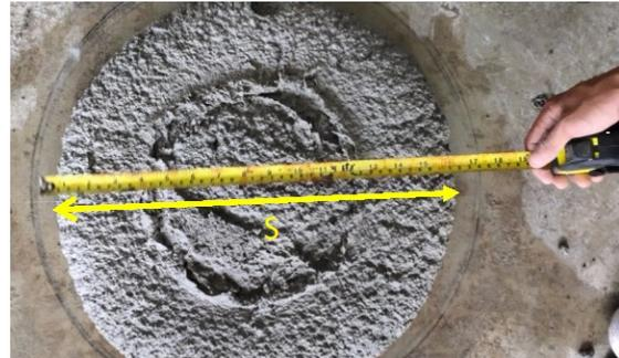
Fig. 5 Slump flow test
