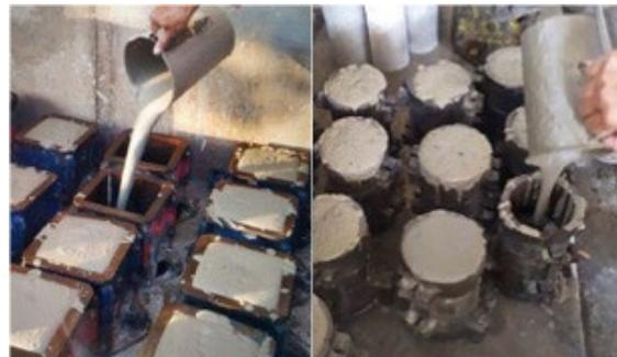
Fig. 4 Casting fresh FC into the mold.
