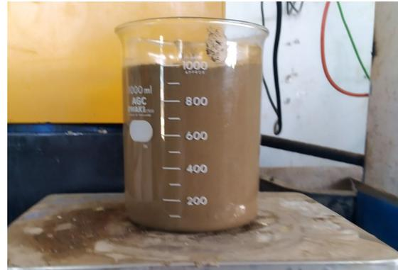
Fig. 3 Wet density testing.
