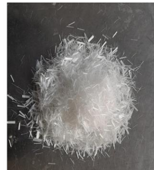
Fig 2. Polyvinyl alcohol (PVA) short fibre
