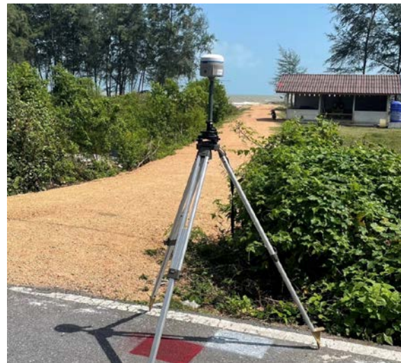
Fig. 5 Rapid static GNSS surveying for CPs
