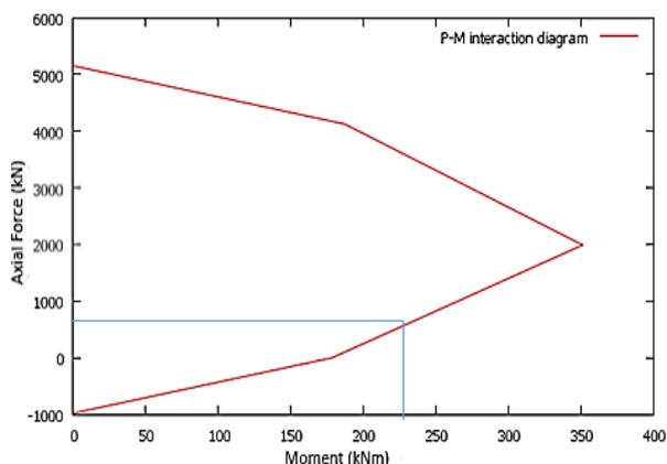
Fig. 7 P-M interaction diagram for second floor C3.
