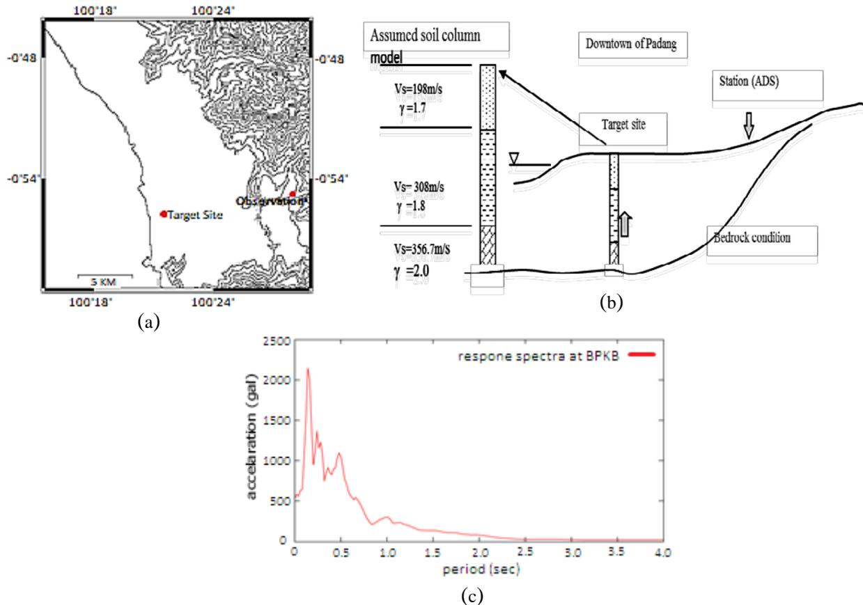
Fig.6 Schematic representation of a procedure for computing effects of local soil conditions on the ground motion: (a) The map of station and target site, red circles are station ADS and BPKP as target site; (b) Schematic representation of procedure; (c) Response spectrum for target site (site BPKP).
