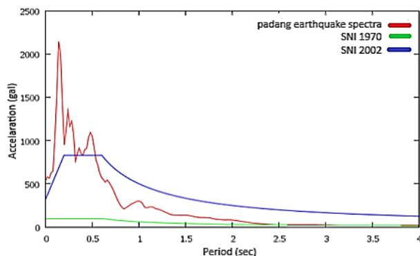
Fig. 1 Comparison of response spectra in each standard; the red line is the current spectra of the Padang earthquake 2009.
