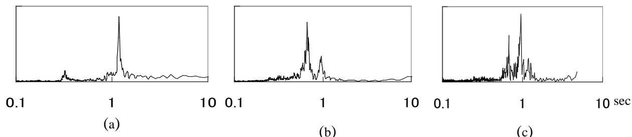
Fig. 5 Predominant period, (a) Sway x=1.19s, (b) Sway y=0.67s and (c) torsion recorded =0.9s on third floor.
