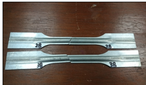
Fig 9 The web stiffeners failure mode.
