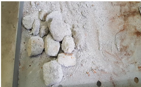
Fig. 11 The example of hardened WBA and WPSA mortar mix after being tested
