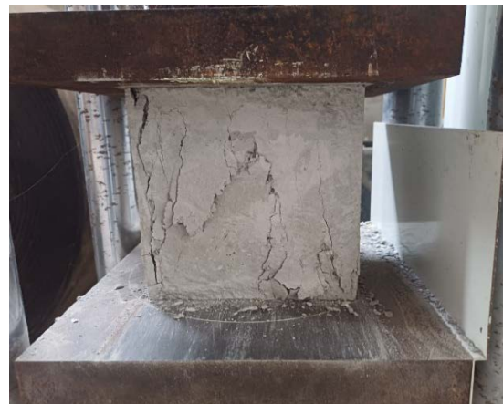
Fig. 5 Concrete compressive strength test specimen
