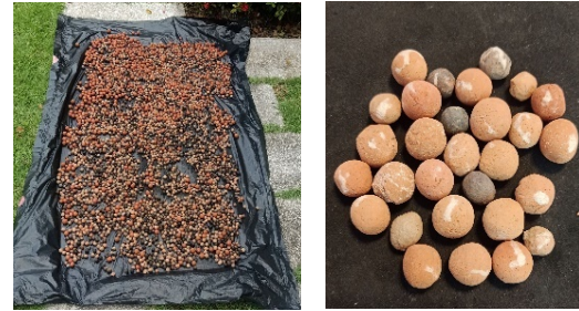
Fig.6 The air-dried fired clay granules with the immobilized microbial cells.
