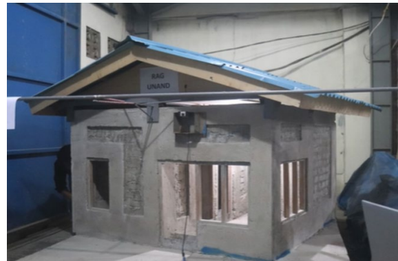
Fig.9 The retrofitted model URM house
