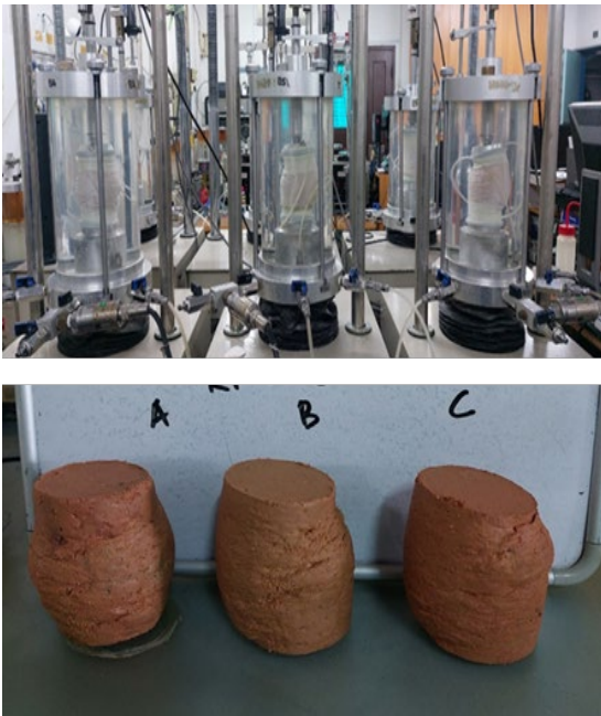
Fig.12 Failed samples after CU triaxial testing
