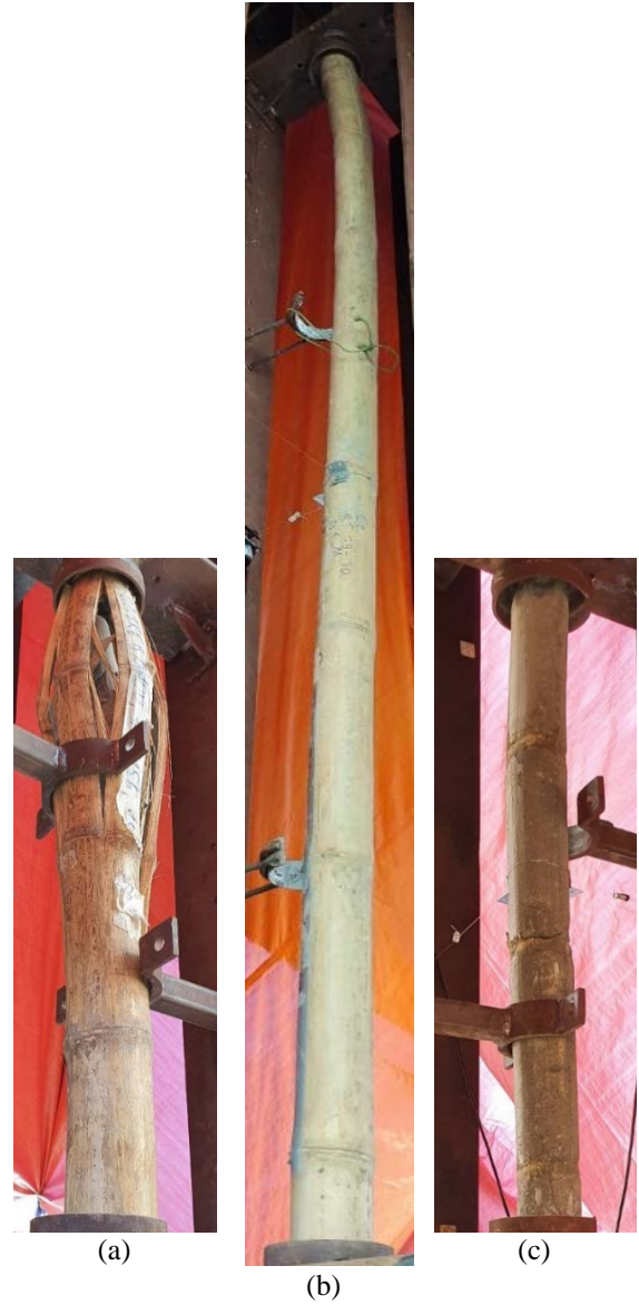
Fig. 5 Failing figure for (a) BC1 sample, (b) BC49 sample, and (c) C8 sample.
