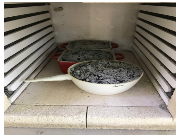
Fig.3 Waste paper ash inside the furnace.
