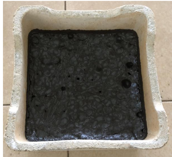
Fig. 4 Bricks fired at 1300 °C completely melted on the alumina saggar
