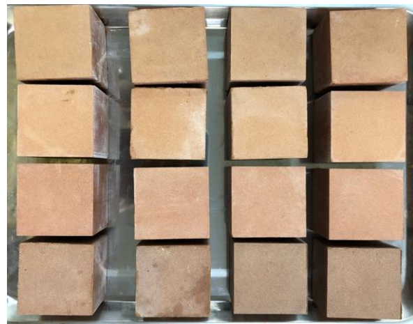
Fig. 2 Fired bricks at 800 °C, 900 °C, 1000 °C, 1100 °C. Bricks are arranged per row with the first row fired at 800 °C; the second row fired at 900 °C, the third row fired at 1000 °C, and the fourth row fired at 1100 °C.
