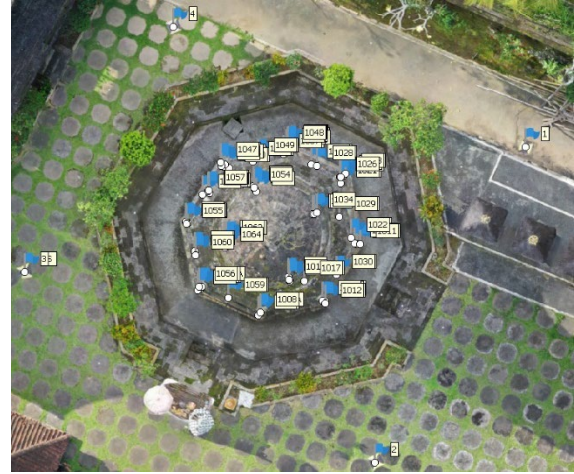
Fig. 3 Distribution of GCP and ICP (a), and measurement of GCP and ICP using RTK-GNSS and ETS (b)
