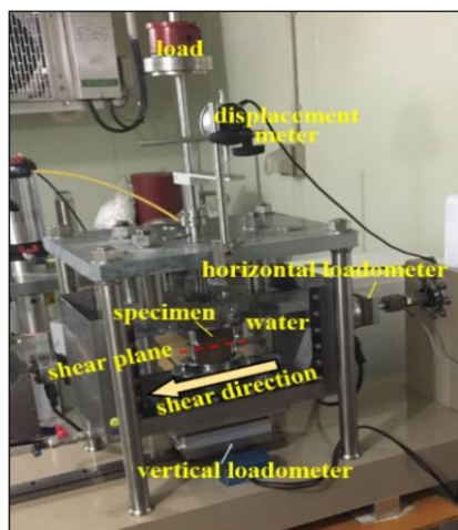
Fig. 3 Direct shear test apparatus
