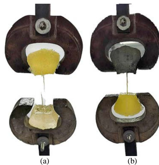
Fig.3 Test setup of fibers in tension testing machine (a) for ultimate tensile load test of a single fiber and (b) for bonding test between fiber and mortar
