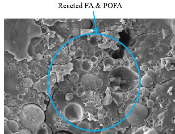
Fig. 10 SEM results for specimens with 10% POFA addition, cured at elevated temperature for 56 days.
