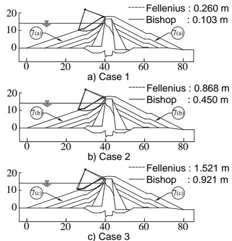
Fig.7 Sliding displacement results with Modified Newmark approach
