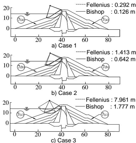
Fig. 6 Sliding displacement results with Conventional Newmark approach
