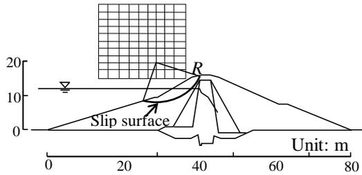
Fig. 5 Circular slip surface in the analysis
