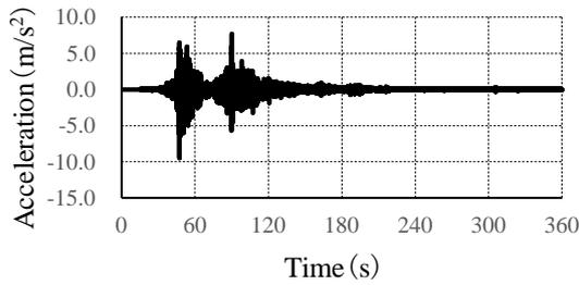
Fig. 4 Acceleration waveform of input motion
