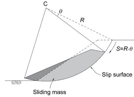
a) Schematic diagram of rotational slide
