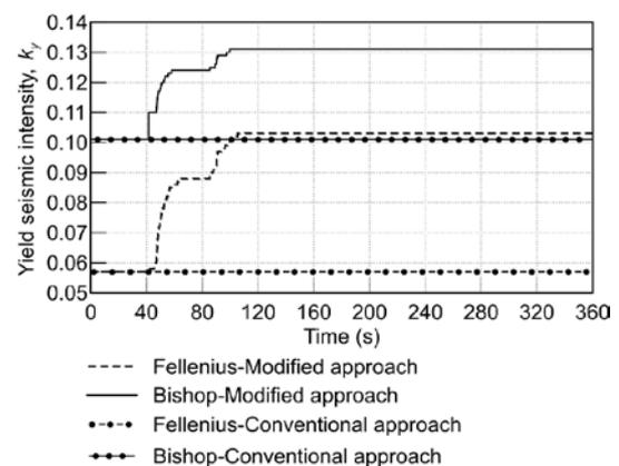
Fig. 9 Yield seismic intensity with time for Case 2
