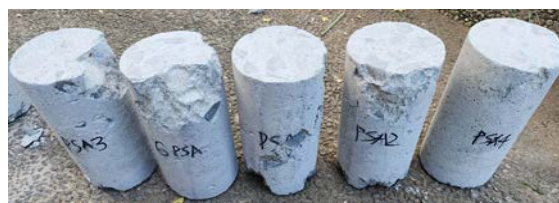
Fig.4 Rupture of concrete specimen containing coated polystyrene aggregates.
