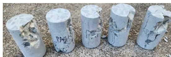
Fig.3 Rupture of concrete specimen containing uncoated polystyrene aggregates.
