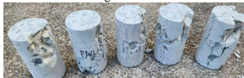
Fig.3 Rupture of concrete specimen containing uncoated polystyrene aggregates.
