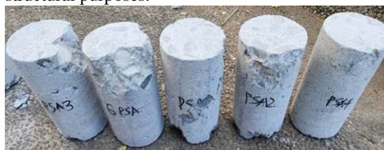
Fig.4 Rupture of concrete specimen containing coated polystyrene aggregates.
