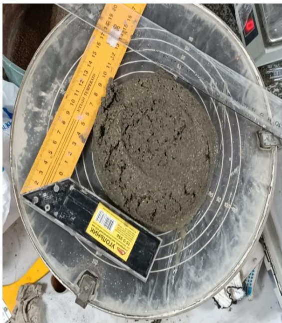
Fig.1 Laboratory testing of specimens, Testing of specimens for cone melting
