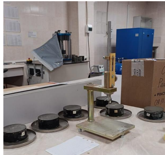
Fig.3 Laboratory testing of specimens, the setting time tests for the cement-sand mixture
