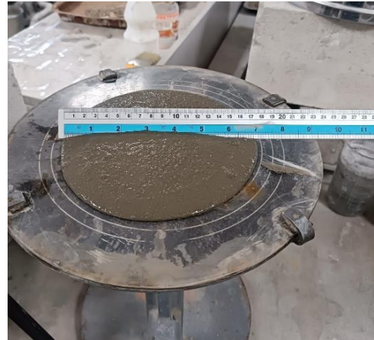
Fig.2 Laboratory testing of specimens, for cone melting
