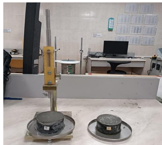
Fig.4 Laboratory testing of specimens. The setting time tests for the cement-sand mixture
