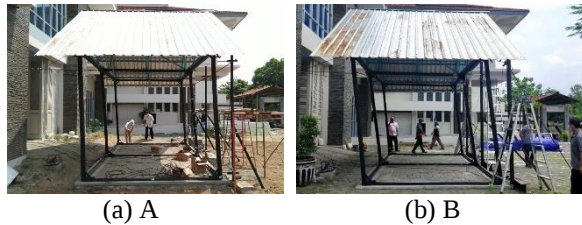
Fig.21 Specimen OF after loading: significant drift without experiencing any structural damage
