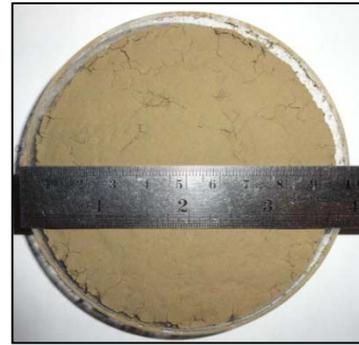
Fig 4. Soil specimen was remolded on a circular plate with 10 mm soil thickness and 100 mm surface diameter.
