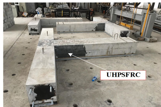
Fig.3 Specimens after removing the formwork
