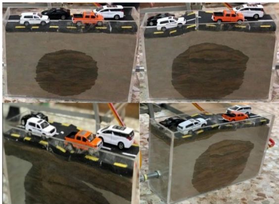
Fig.9 Progress of sinkhole occurrence in the stabilized sand bed.
