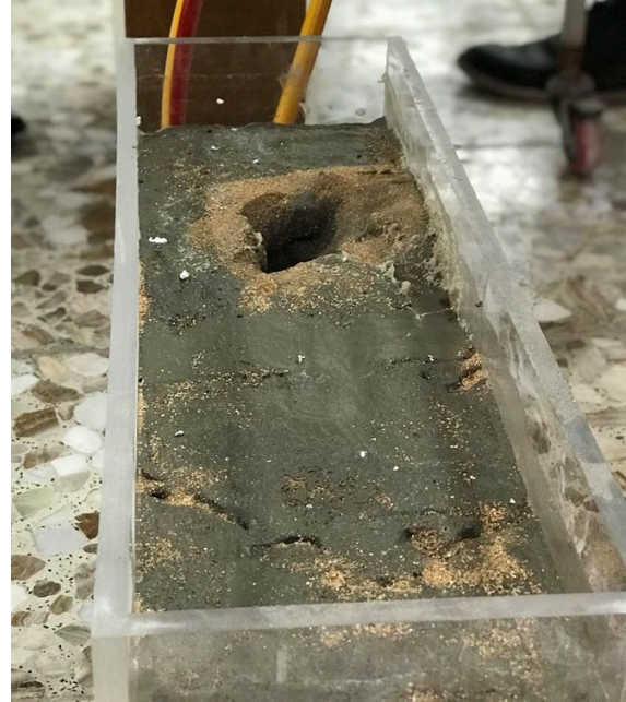
Fig.11 Sinkhole occurred in the stabilized sand bed.
