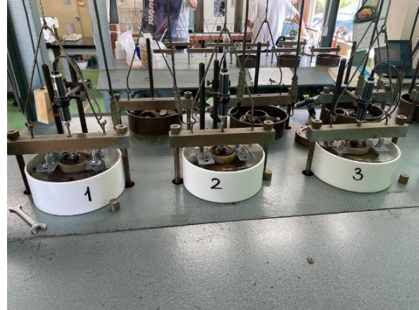
Fig. 8 Swell potential and swell pressure test of soil Specimens
