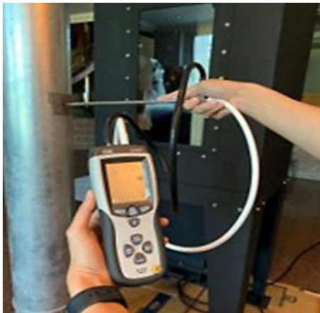
Fig. 5 Measurement of the exhaust air velocity at location V3.
