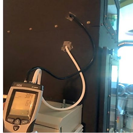
Fig. 6 Measurement of the pressure drop within the baghouse.
