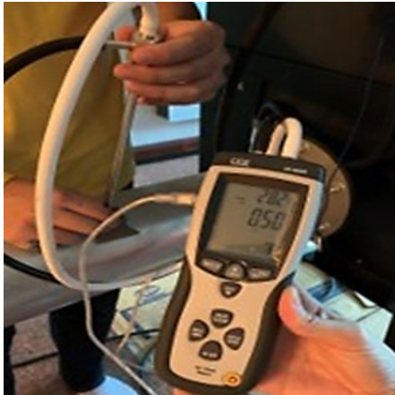
Fig. 4 Measurement of the inlet air velocity at location V2.
