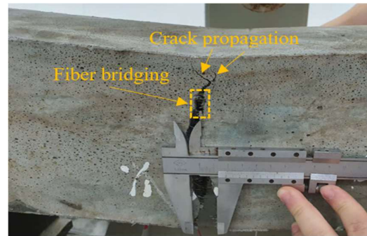
Fig. 2 Effect of steel fiber on crack propagation
