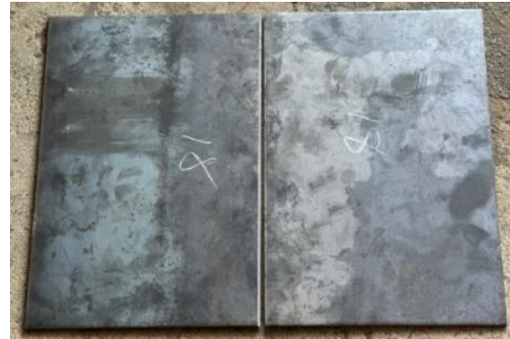
Fig. 2 Actual Unwelded Test Coupon with V-groove Butt Joint
