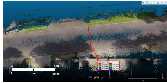
Fig. 7 Road Width using TLS
