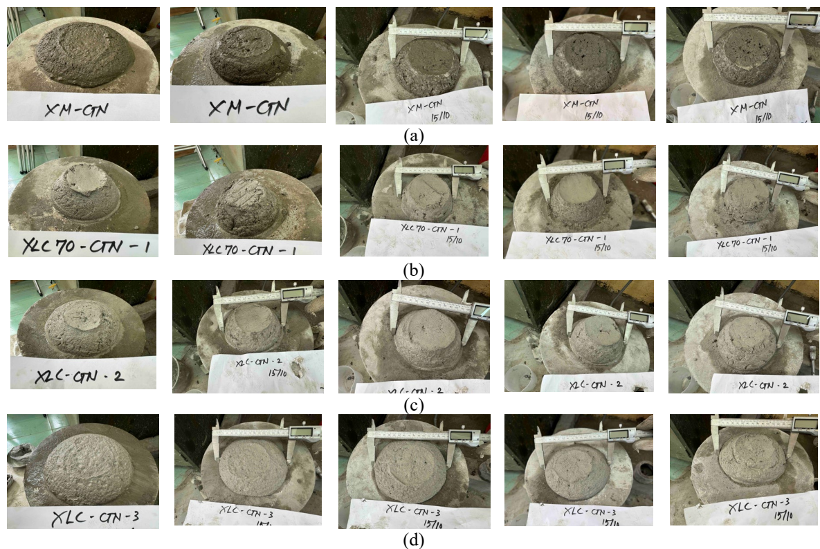
Fig. 5 Experiment for workability loss of mortar specimens (a) PC-NS; (b) GGBFS-NS-1; (c) GGBFS-NS-2; (d) GGBFS-NS-3
