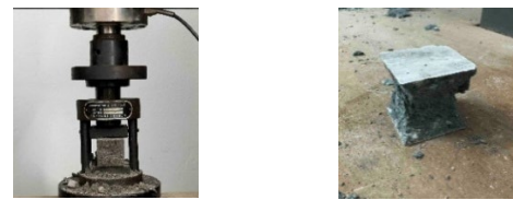
Fig. 8 Compressive strength experiment for mortar specimens
