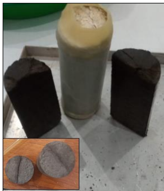
Fig. 8. Soil sample after crack modeling.
