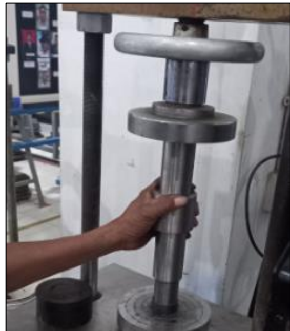
Fig. 7. A pressure tool to create cracks in soil samples.
