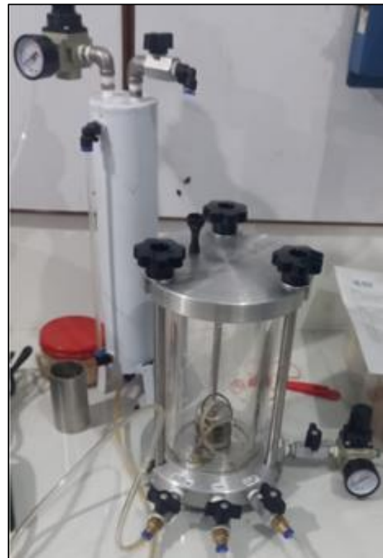
Fig. 5. Photo of infiltration modification test tool on cracked soil.
