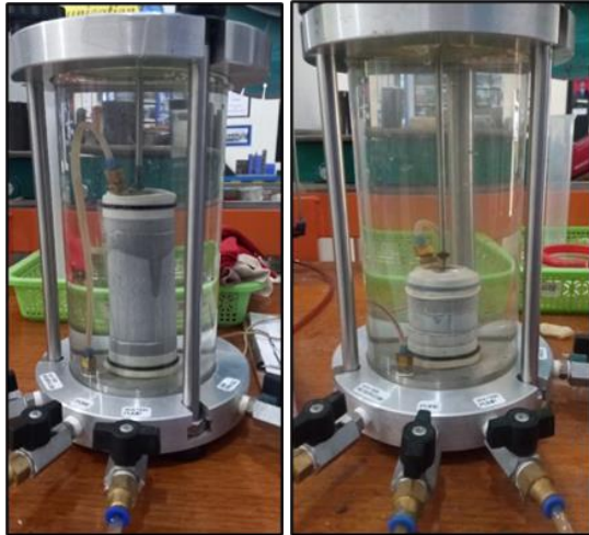
Fig. 9. The process of draining water into cracked soil samples with different heights.
