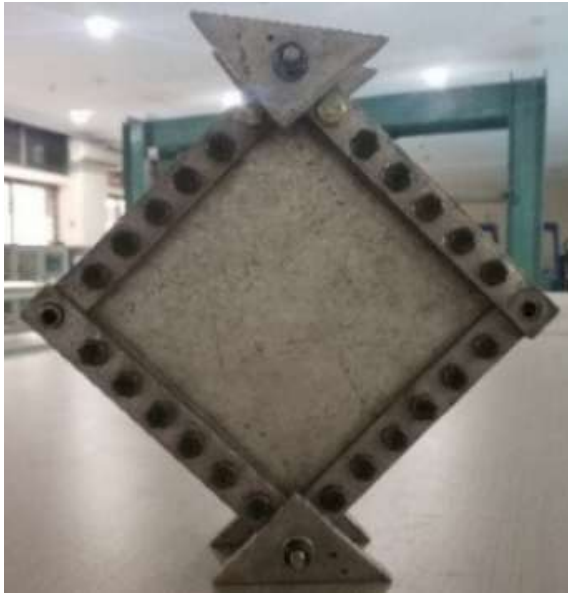
Fig. 7 Pure shear plate test specimen
