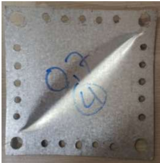
Fig. 12 Representative conditions after 0.7 mm thick plate test
