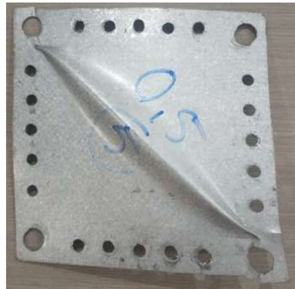
Fig. 10 Representative conditions after 0.5 mm thick plate test
