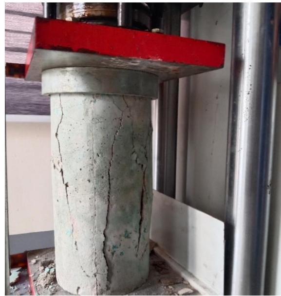
Fig.4 Sample testing using a compressive machine
