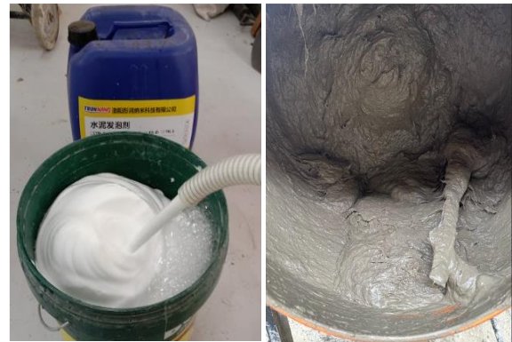
Fig.2 Preparation of foamed concrete with coir fiber: (a) the generated foam and (b) the foamed concrete with coir fiber.
