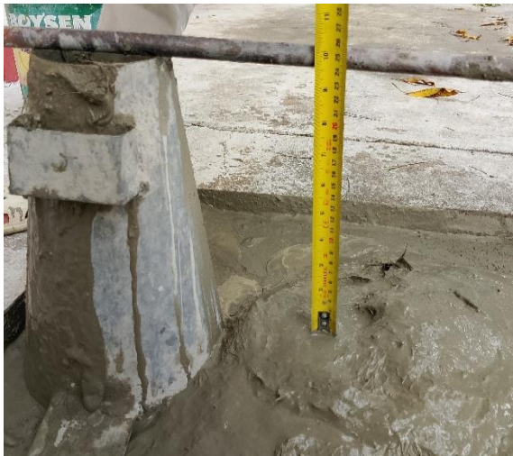
Fig.3. Slump flow test of foamed concrete.
