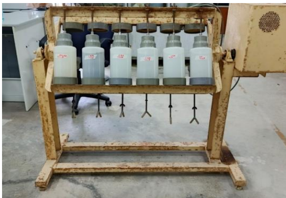
Fig. 6 Agitation of concrete sample during leaching test (SPLP method)
