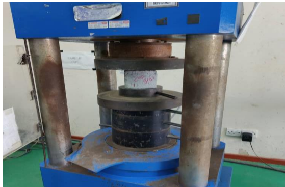
Fig.5 Testing of concrete cubes under compression using a universal machine
