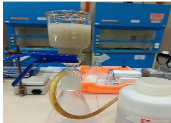
Fig.7 Filtration of leachate through 0.7 \mu\text{m} glass fiber
