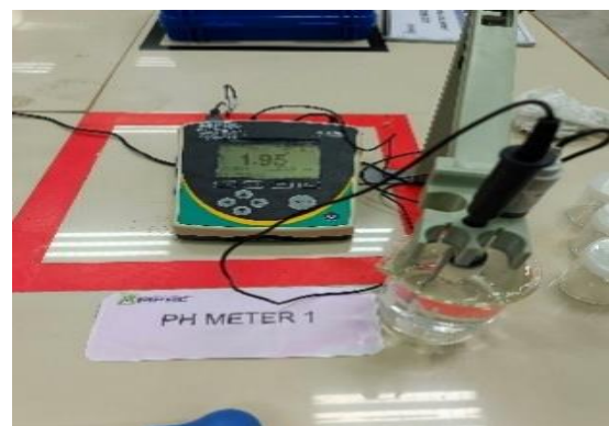
Fig. 8 pH adjustment of filtered leachate prior to ICP-MS analysis.
