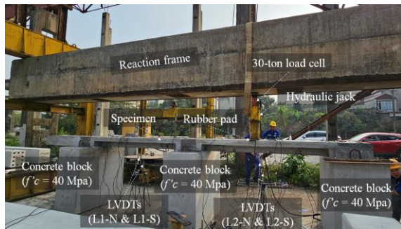
Fig. 10 Load cell and LVDT placement
