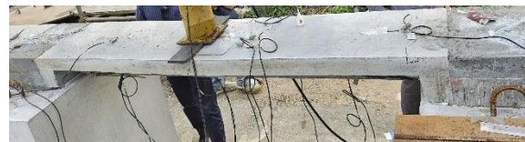
Fig. 19 Connection was maintained after failure
