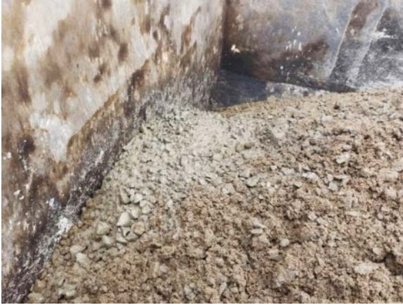
Fig.9 The cement paste was not evenly distributed and tended to accumulate on one side
