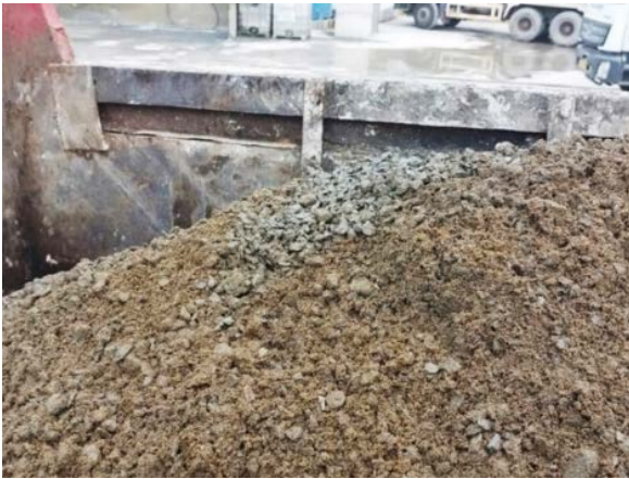
Fig.10 The aggregate, cement, and fly ash were not uniformly mixed during large-scale mixing
