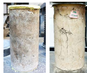
Fig.3 Visual inspection of RCC using 50/50 and 60/40 fraction of gravel/sand
