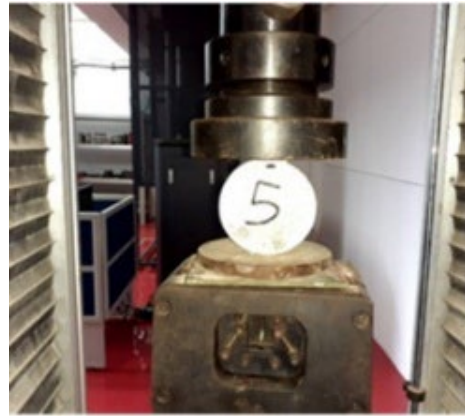
Fig. 4 Sample of a pre-loaded concrete specimen, showing specimen #5
