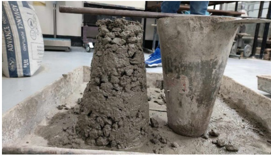
Fig. 2 Slump Tests of Cement
