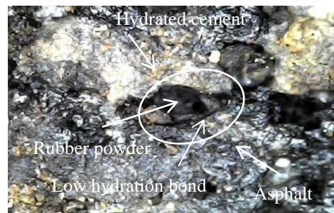
Fig.5. Rubber powder bond failure on the CAM (x100)
