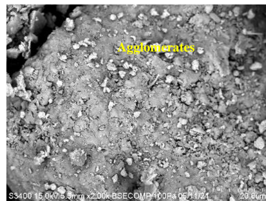
Fig.7b Microstructural image of Treated DOBE at 20 \mu\text{m} magnification
