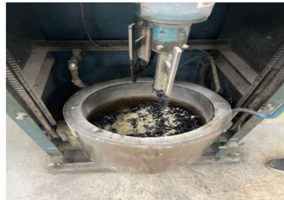
Fig. 1 Preparation of stone mastic asphalt sample with capsules.
