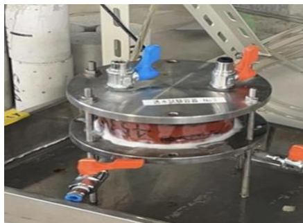
Fig. 10 Status of Lab permeability test
