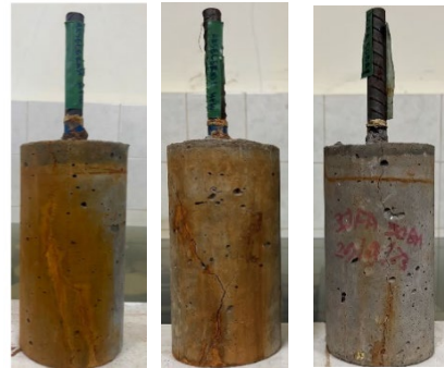
Fig. 8 Visual condition of specimens after corrosion acceleration test (left to right: Control specimen (C), 15%FA50%BA, 30%FA50%BA)
