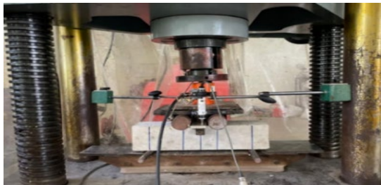
Fig. 3 Flexural strength test setup using the two-point loading method
