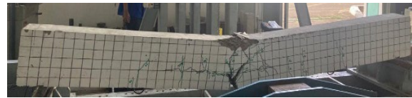
Fig. 8 Crack pattern of specimen B-UHPC 50
