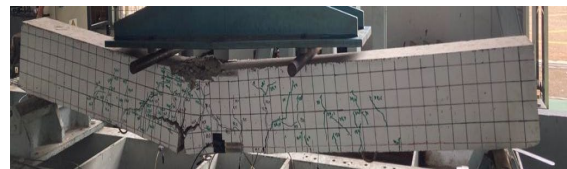
Fig. 6 Crack pattern of specimen B-UHPC 15
