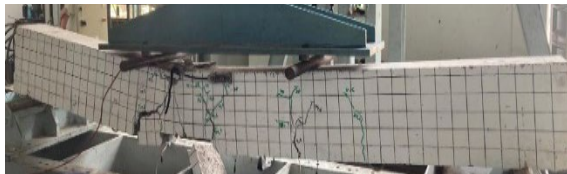
Fig. 5 Crack pattern of specimen B-N 50
