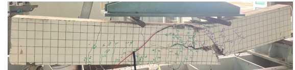
Fig. 9 Crack pattern of specimen B-UHPC 70.
