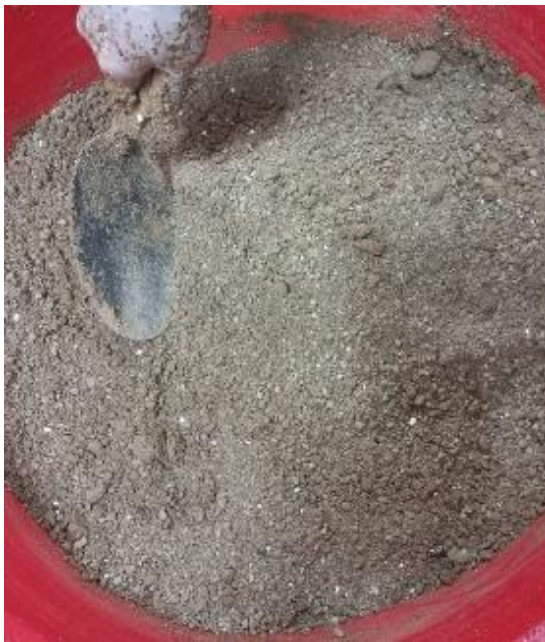
Fig. 2. Mixture of clay and 6% marble ash
