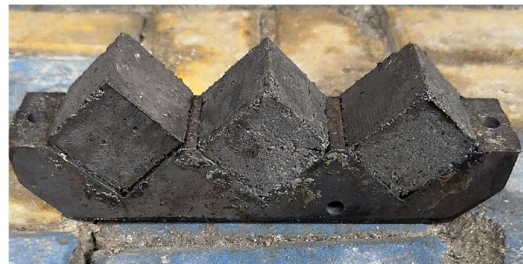
Fig.1 Fly-ash based geopolymer mortar specimens
