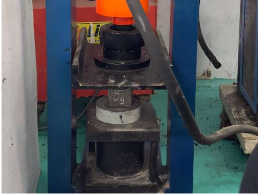
Fig.3 Unconfined Compression Strength (UCS) test
