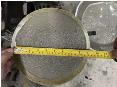
Fig. 3 Flow Table Test
